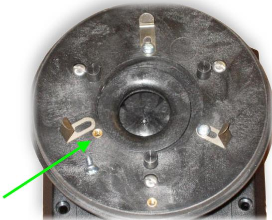
Care must be taken not to over-tighten or cross-thread any of the screws. The tool required is a small Pozi-head screwdriver (Cantium Scientific Limited part number P0001SCRD). If any screws are lost, they can be replaced with Cantium Scientific Limited part number P0001SCR003.
