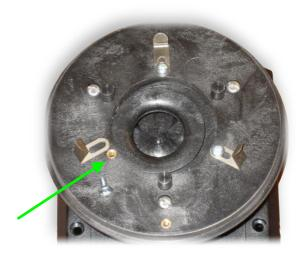
Care must be taken not to over-tighten or cross-thread any of the screws. The tool required is a small Pozi-head screwdriver (Cantium Scientific Limited part number P0001SCRD). If any screws are lost, they can be replaced with Cantium Scientific Limited part number P0001SCR003.
